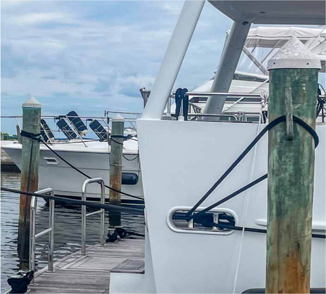
Looping dock line around a pile and belaying both ends on the boat makes it easier to remove the line and take it with you.
